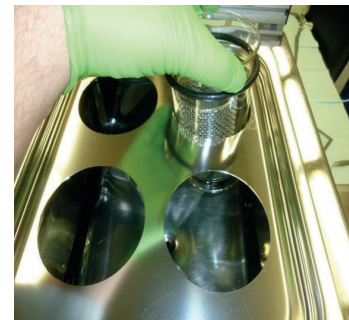
Place beaker in ultrasound bath
