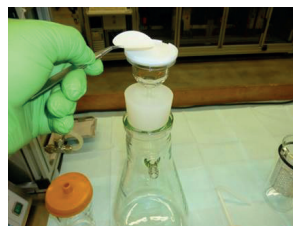
Place filter in filtration unit
