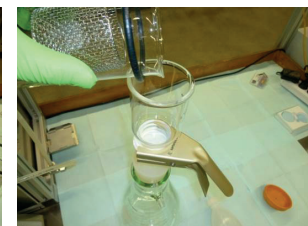
Empty beaker into filtration unit
