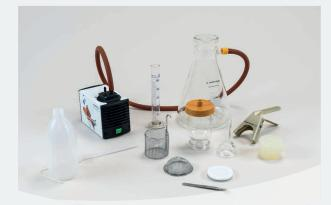
**Basic equipment** to the cleaning and extraction of components to VDA Bd. 19. Optionally ultrasonic trays and drying devices are offered, according to component size. We like to advice you individually.
