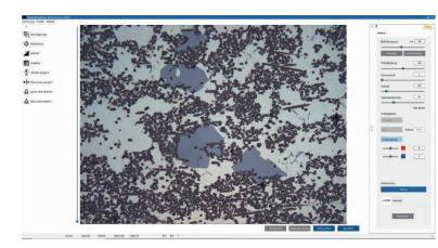
4 image sources with their own additional modul can be controlled directly on a PC. The live image remains open in the background and is automatically closed when another image source is called up.
