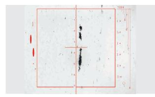
Manual analysis is particularly suitable **for tests based on the mean value (such as the DIN 50602 K methods).** Depending on the type of steel, only a low number of inclusions are analysed as part of methods such as K3 and K4.
